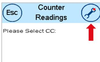
Counter Readings: Select the spanner in the top right of screen.
